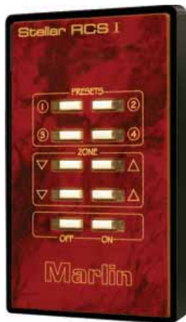
RCS I with 4 presets, 2-zone raise/lower, and master on/off
